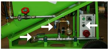
**10.** Get in the habit of always emptying the entire system of water by opening both blue taps and holding down the **Water** (Vatten) button.
