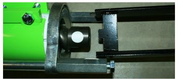
**11.** Fit the mixer shaft, ensuring it is in the correct position in the rotor.
