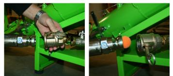
**1.** Remove the hose and put in a cleaning ball and connect the hose to the plugged water outlet on the pump.
