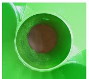
**7.** Check the mixing pipe on the pump and scrape any deposits.
