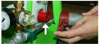
**6.** Plug the power cord 3 phase 400V to the connector on the electric cabinet (left side).
