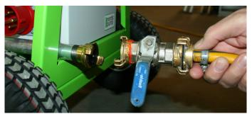
**5.** Connect the water to the clutch connector on the back of the pump.
