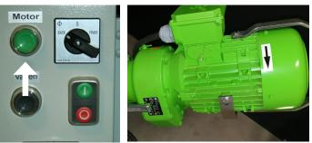
**9.** Press the **Motor** button on the electric cabinet and check that the engine is in the right direction, the engine should rotate counterclockwise, see the arrow on engine hood.
