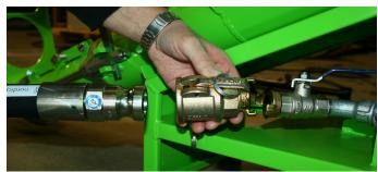
**13.** Connect the pump hose to the water outlet on the pump and fill approximately five liters of water and then connect the hose to the pump.
