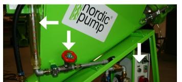
**7.** Press the **Water** (Vatten) button to adjust the amount of water in the measuring pipe. The amount of water is read at the top of the cone.
