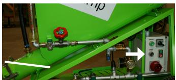
**14.** Press the **WATER** button and fill water in the mixing chamber.
