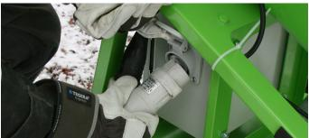
**9.** Connect the remote control cable to the gray jack on the right side.
