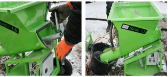
**6.** Unscrew the rotor with the t-handle and remove the mixer shaft and clean it from the screeds residue.
