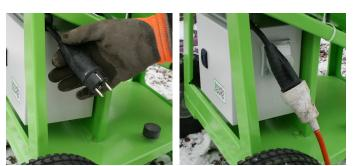
6. Connect the power cord to the electric socket.
