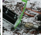
**10.** Fill the pump hose with 3 - 5 liters of water with the supplied hose clutch and then connect the hose to the pump.
