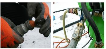
**3.** Remove the hose and put in a cleaning ball and connect the hose with the supplied hose clutch to the water outlet on the front of the pump.
