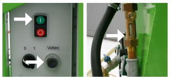
**7.** Set the pump to the starting position by pressing the green button on the electric cabinet.
