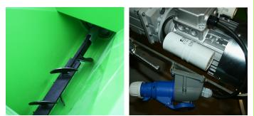
**3.** Fold up the engine and insert the carrier against the mixing shaft, connect the power cord to the motor.
