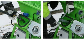
**2.** Fold the engine and spray the rotor with silicone spray and screw in the rotor in the stator with the t-key and the mixer shaft.
